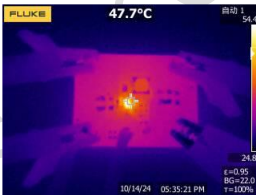
Figure 19. Thermal, V_{IN}=5V, V_{OUT}=1.2V, I_o=2A (TTBR)
