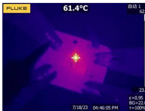
Figure 20. Thermal, V_{IN}=5V , V_{OUT}=1.2V , I_{LOAD}=3A
