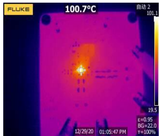
Figure 22. Thermal, 12 VIN, 1 Vout, 8A
