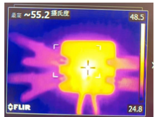
Figure 20. Thermal, 12VIN, 3.3Vout, 3A(SOT563)
